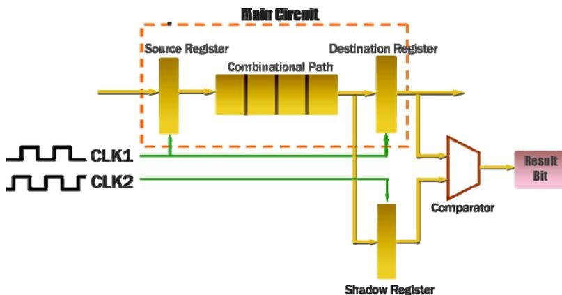
Figure 2. Delay characterization with negative-skewed shadow register [5]
