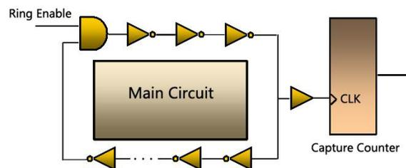
Figure 3. Ring-oscillator temperature monitor
