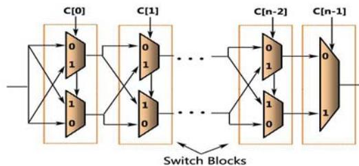
Figure 1. A typical PUF delay circuit
