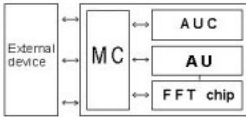
Fig. 1. Scalable EC architecture with FFT chip
