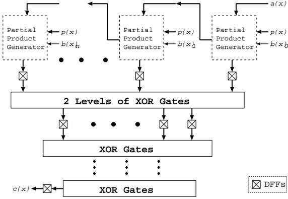
Fig. 3. Block diagram of pipelined FPGA implementation
