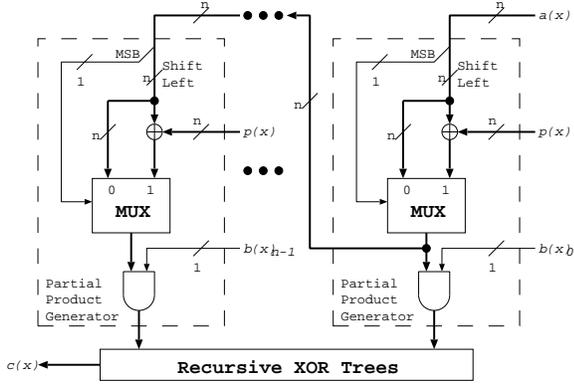
Fig. 1. Block Diagram of recursive implementation. Note that the result of each partial product module is fed into the next.
