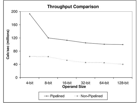
Fig. 4. Pipelined performance does not include cold start
