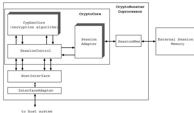
Fig. 1. Block diagram of CryptoBooster architecture.
