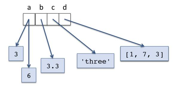
The object (3) referred to by variable a does not change; instead, a refers to a new object (6)
